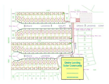
Because Drake Landing Solar Community is using a lower water temperature than most district heating systems, it was necessary to more carefully engineer the in-home heating system. For instance, domestic hot requires a minimum of 60 degrees Celsius and space heating requirements are lower. The economics and engineering indicated we should install independent solar hot water systems in each home.
